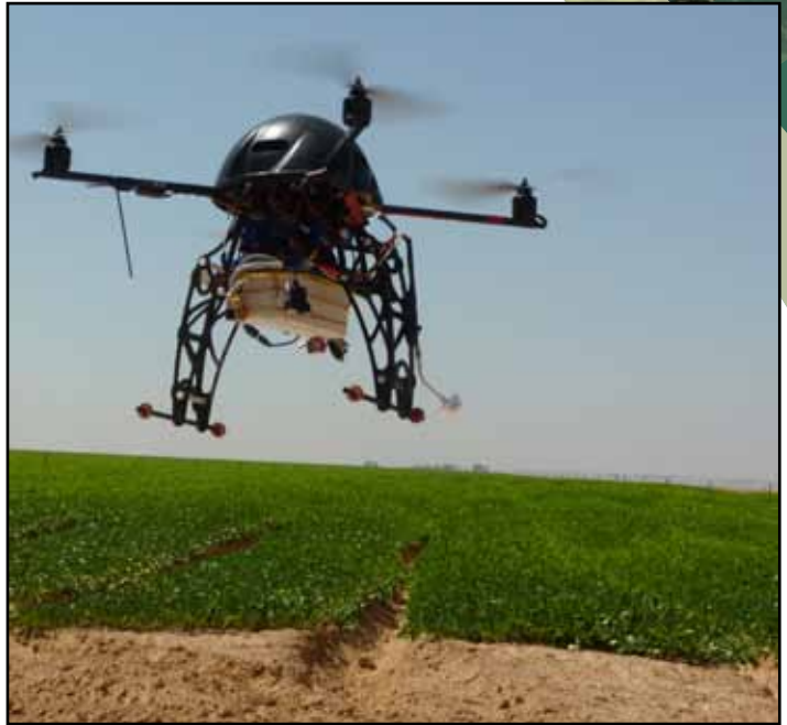
A Robin camera mounted on a quad-copter hovering over a peanut field in the South of Israel.
